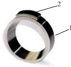
Fig. 1. The sliding pair; 1-annular sample, 2-counter-sample
