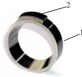
Fig. 1. The sliding pair; 1-annular sample, 2-counter-sample
